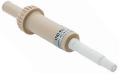
LARGE PIPETTOR (1 mL)
